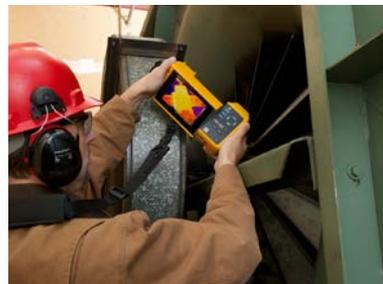
**Get tough shots from any angle with a 240° degree rotating lens and the only 5.7 inch LCD.**
