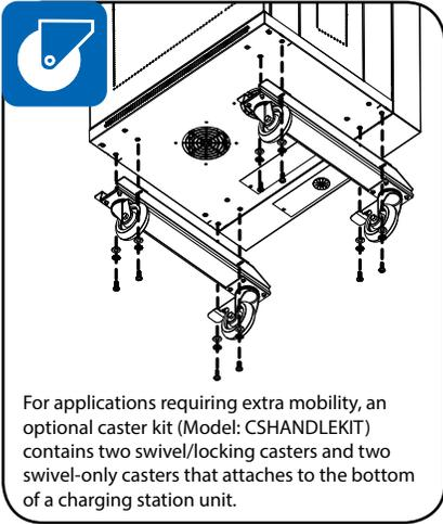
For applications requiring extra mobility, an optional caster kit (Model: CSHANDLEKIT) contains two swivel/locking casters and two swivel-only casters that attaches to the bottom of a charging station unit.
