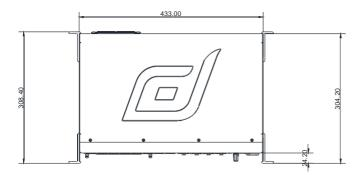
CDM64 - without box Width - 481.6mm/19" Depth - 309mm/12.2" Height - 354.5mm/14"/8U Weight - 13.5kg/29.7lbs
